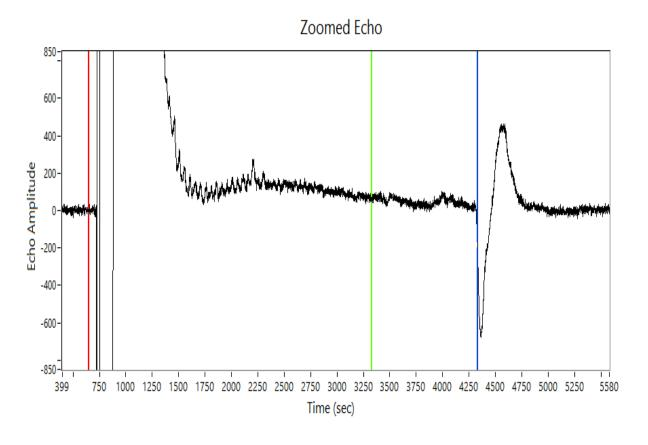
Depth: 1147.00 ft Return Time: 3.68 sec Acoustic Velocity: 623.20 ft/s Average Joint Length: 31.00 ft Number of Joints: 37.00
