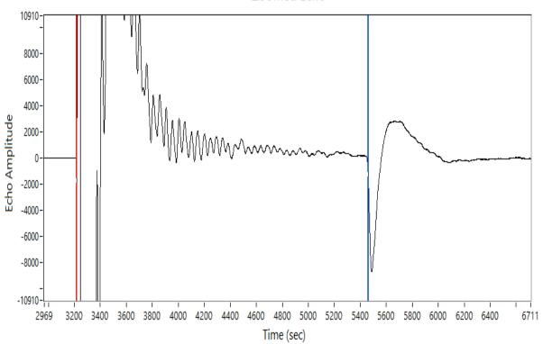
660.00 ft Depth: Return Time: 2.24 sec Acoustic Velocity: 588.76 ft/s Average Joint Length: 30.00 ft Number of Joints: 22.00
