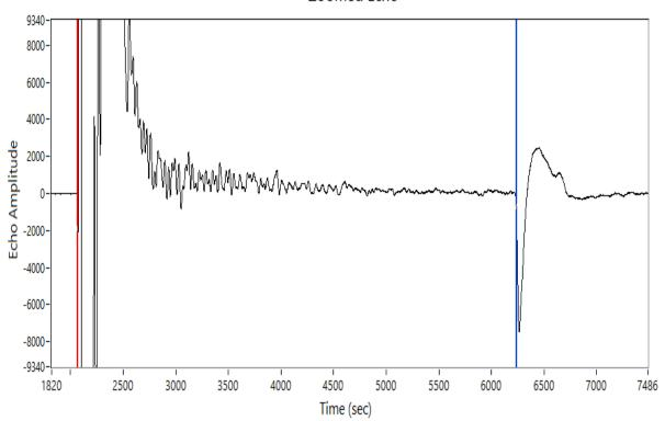
Depth: 1950.00 ft Return Time: 4.17 sec Acoustic Velocity: 936.15 ft/s Average Joint Length: 30.00 ft Number of Joints: 65.00
