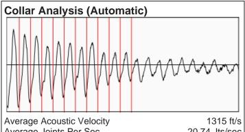
Average Joints Per Sec. 20.74 Jts/sec Joints To Liquid 81.89 Jts
