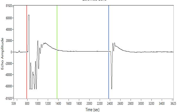
1147.00 ft Depth: Return Time: 1.59 sec Acoustic Velocity: 1446.41 ft/s Average Joint Length: 31.00 ft Number of Joints: 37.00
