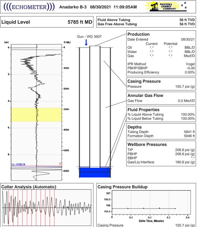
Average Acoustic Velocity Average Joints Per Sec. 20.51 Jts/sec Joints To Liquid 182.18 Jts
