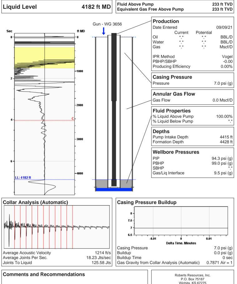
Fluid Level for TA. CP=7 psig. Tubing Leak @ 1320'
