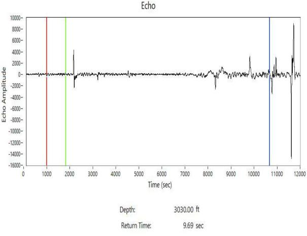
Acoustic Velocity: 625.52 ft/s Average Joint Length: 30.00 ft Number of Joints: 101.00
