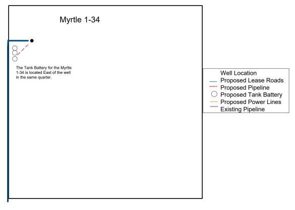
Proposed Details of SW/4 Sec 34 – T23S – R35W
