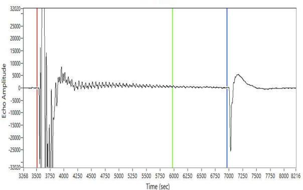
1380.00 ft Depth: Return Time: 3.45 sec Acoustic Velocity: 800.46 ft/s Average Joint Length: 30.00 ft Number of Joints: 46.00
