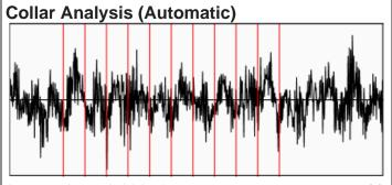
Average Acoustic Velocity Average Joints Per Sec. Joints To Liquid 1120 ft/s 17.67 Jts/sec 162.32 Jts
