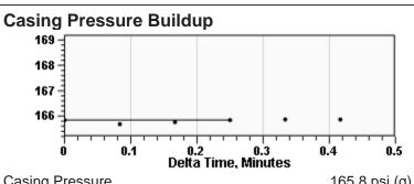
Casing Pressure 165.8 psi (g) Buildup -0.0 psi (g) **Buildup Time** 15 sec Gas Gravity 0.8028 Air = 1
