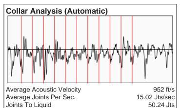
54.5 54 53.5 Delta Time, Minutes Casing Pressure 53.7 psi (g) Buildup -0.1 psi (g) **Buildup Time** 2 min 0 sec 0.9986 Air = 1Gas Gravity from Collar Analysis (Automatic)
