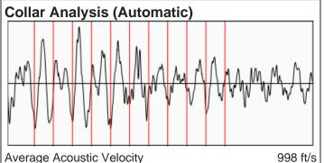
Average Acoustic Velocity Average Joints Per Sec. Joints To Liquid 998 ft/s 15.78 Jts/sec 88.10 Jts
