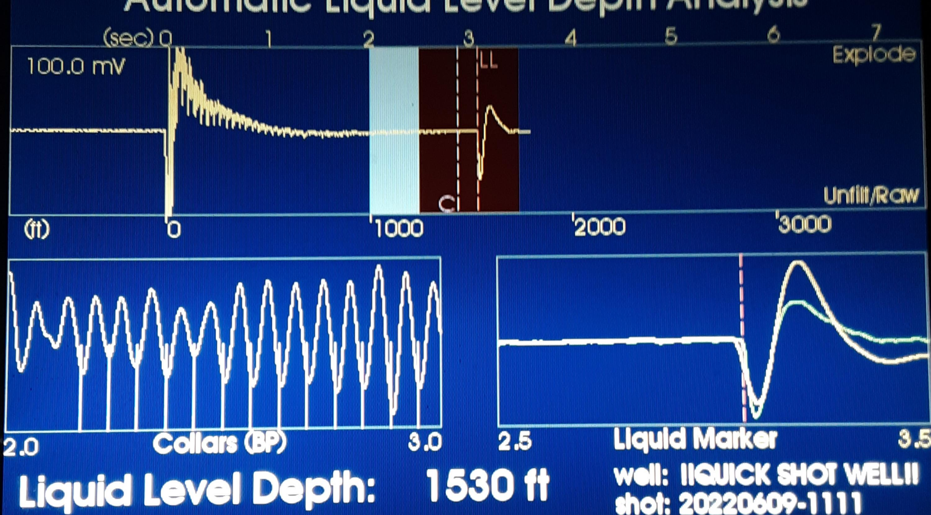
Joints to Liquid Level: 48.27 Time to Liq Lev (sec): 3.066
