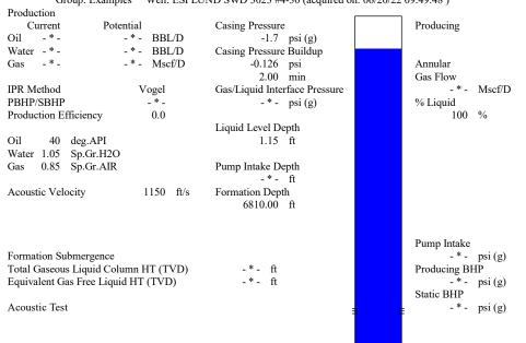
Entered Acoustic Velocity for Liquid Level depth determination
