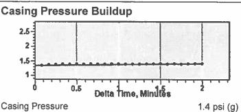
Buildup 0.1 psi (g) **Buildup Time** 2 min 0 sec Gas Gravity from Acoustic Velocity  $0.8433 \, Air = 1$
