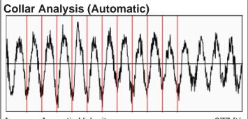
Average Acoustic Velocity Average Joints Per Sec. Joints To Liquid 977 ft/s 15.41 Jts/sec 119.90 Jts
