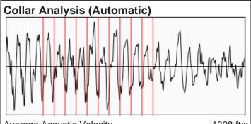
Average Acoustic Velocity Average Joints Per Sec. Joints To Liquid 1398 ft/s 22.70 Jts/sec 148.05 Jts
