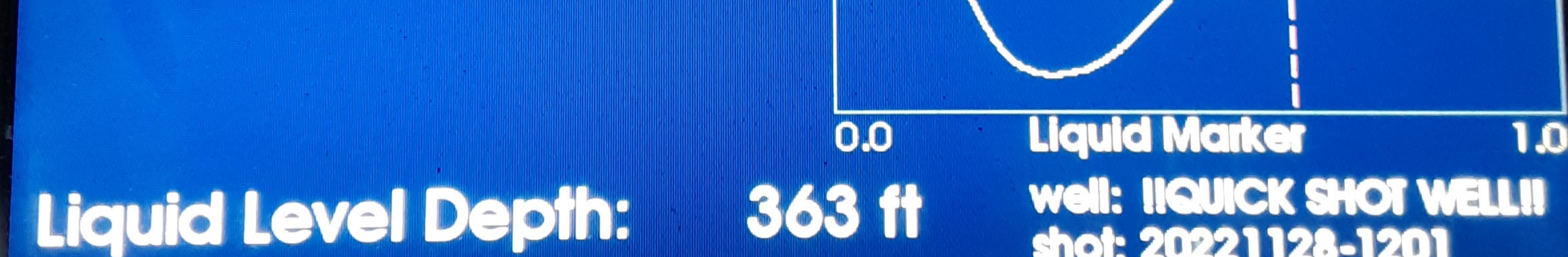
Joints to Liquid Level: 11.45 Avg Jts/sec: 18.14 Avg Jt Len: 31.70 ft Time to Liq Lev (sec): 0.631 Average Acoustic Velocity: 1150 ft/sec
