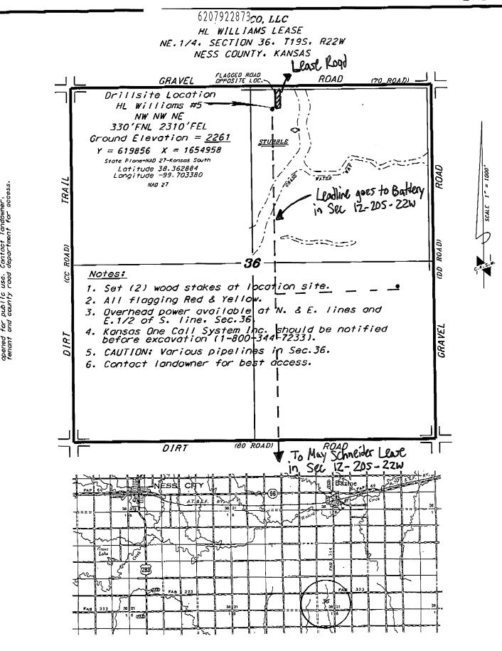
Controlling dots is based upon the best maps and phatographs available to us and upon a regular section at land containing 640 occus.
