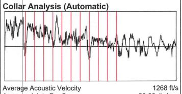
Average Acoustic Velocity Average Joints Per Sec. Joints To Liquid 1268 ft/s 20.00 Jts/sec 117.18 Jts
