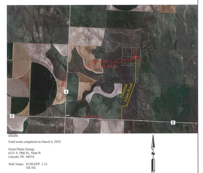
Well Location: Section 13, T5S, R42W, Cheyenne County, Kansas 660' FNL and 330' FEL Ground Elevation = 3619.2 Ngvd '29 Lat. 39°37'27.55" Long. -101°58'35.35" NAD83
