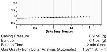
Casing Pressure Buildup
