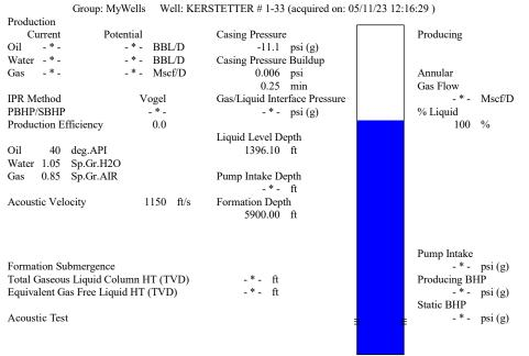
Entered Acoustic Velocity for Liquid Level depth determination
