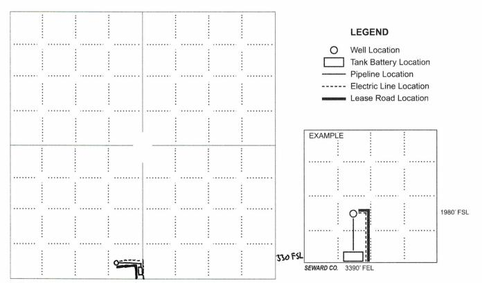
NOTE: In all cases locate the spot of the proposed drilling locaton. 2204 FWL
