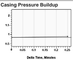
$\begin{array}{lll} \text{Casing Pressure} & 0.8 \text{ psi (g)} \\ \text{Buildup} & 0.1 \text{ psi (g)} \\ \text{Buildup Time} & 15 \text{ sec} \\ \text{Gas Gravity} & 0.9275 \text{ Air} = 1 \\ \end{array}$
