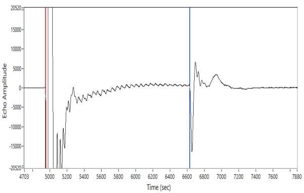
Depth: 930.00 ft 1.68 sec Return Time: Acoustic Velocity: 1109.12 ft/s Average Joint Length: 31.00 ft Number of Joints: 30.00
