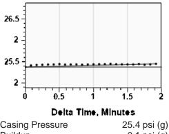
Buildup 0.1 psi (g) Buildup Time 1 min 55 sec Gas Gravity 0.7331 Air = 1
