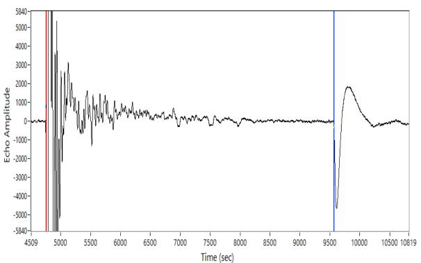
Depth: 2449.00 ft Return Time: 4.81 sec Acoustic Velocity: 1018.30 ft/s Average Joint Length: 31.00 ft Number of Joints: 79.00
