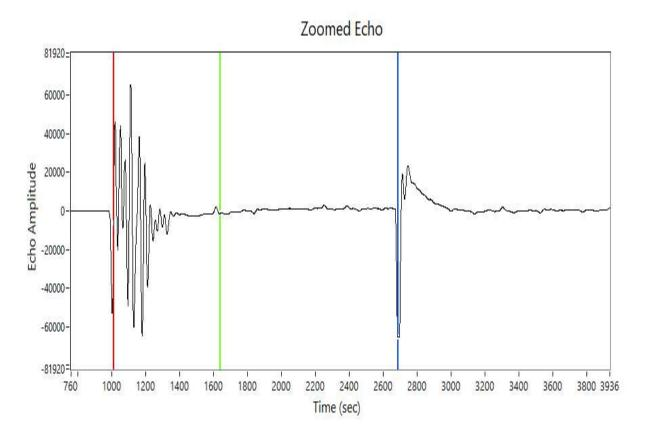
Depth: 1178.00 ft Return Time: 1.68 sec Acoustic Velocity: 1405.73 ft/s Average Joint Length: 31.00 ft Number of Joints: 38.00
