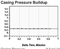
$\begin{array}{lll} \text{Casing Pressure} & 0.3 \text{ psi (g)} \\ \text{Buildup} & -0.0 \text{ psi (g)} \\ \text{Buildup Time} & 50 \text{ sec} \\ \text{Gas Gravity} & 0.7655 \text{ Air} = 1 \\ \end{array}$
