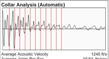
Average Joints Per Sec. 19.64 Jts/sec Joints To Liquid 64.95 Jts
