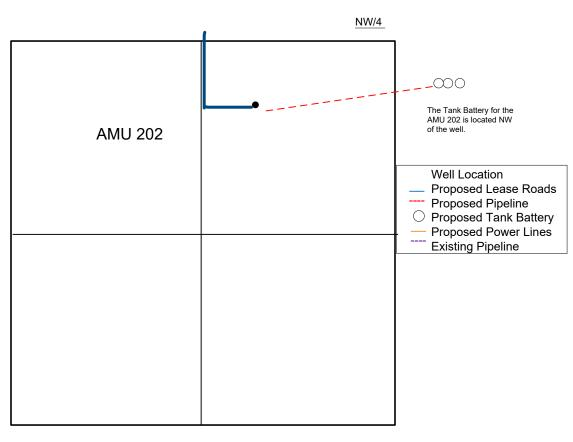
Proposed Details of NW/4 Sec 4 – T27S – R33W
