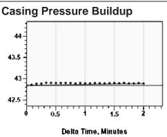
Casing Pressure 42.8 psi (g) Buildup 0.0 psi (g) Buildup Time 2 min 0 sec Gas Gravity 0.7215 Air = 1
