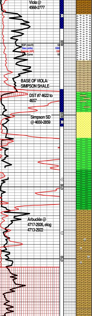
4580 40 min: Heavy oil odor from the sample, Dolomite: fine granular, brown, fair to poor intergranular porosity, fair to good cut, fair show of free oil when chrushed under black light. Chert: dark brown, blocky slow cut.
