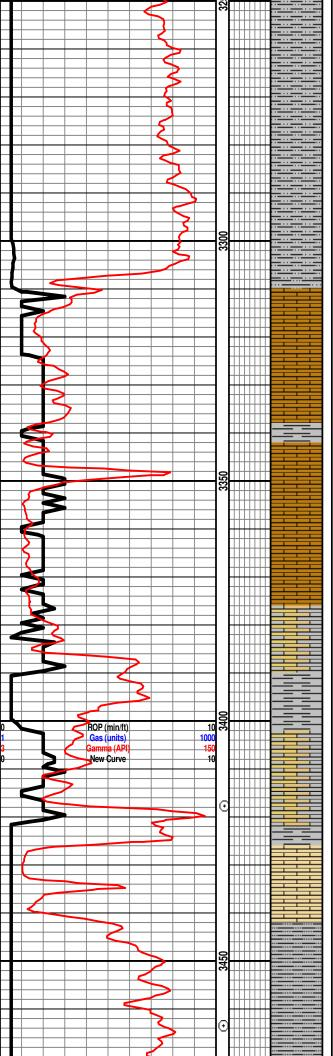
3274: flood of silty micaceous shale with dense siltstone layers dense poor intergranular porosity, shaley no show of gas bubbels, light gray very dense, no show, no fluorescence
