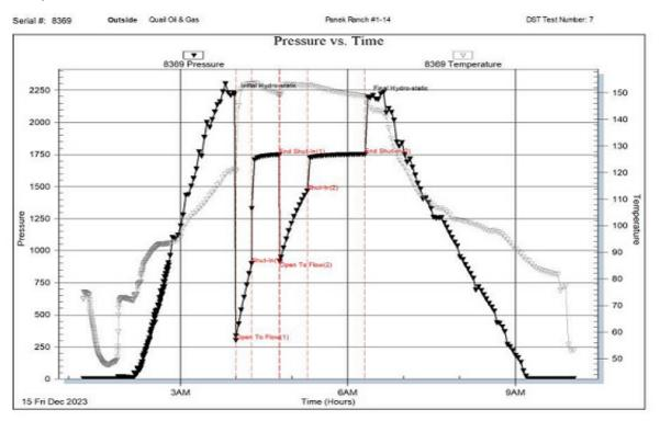
DST (8) 4523 to 4590, Viola straddle test after Elog: IFP Weak blow building to 3.4", ISIPNo blow back, FFP: Weak building blow built to 2.57", FSIP: No blow back, REC 10 mud 100% mud, 121 GIP, IHP 2267 to 2008#, BHP 254 to 189#, IFP 50 to 49, FFP 45 to 55.9#, BHT
