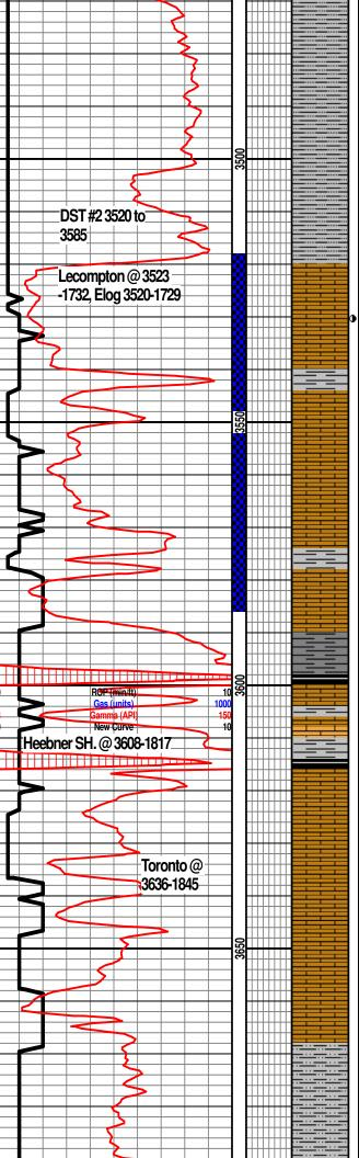
3463 20 min: Siltstone: gray, fine grain, friable no fluoresence, dense, poor intergranular porosity, no show of gas
