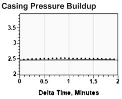
$\begin{array}{lll} \text{Casing Pressure} & 2.5 \text{ psi (g)} \\ \text{Buildup} & 0.0 \text{ psi (g)} \\ \text{Buildup Time} & 1 \text{ min 55 sec} \\ \text{Gas Gravity} & 0.7040 \text{ Air} = 1 \\ \end{array}$
