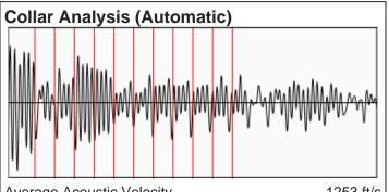
Average Acoustic Velocity Average Joints Per Sec. Joints To Liquid 1253 ft/s 19.76 Jts/sec 88.17 Jts
