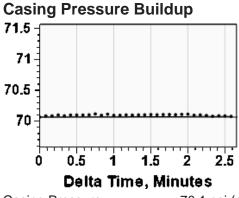
$\begin{array}{lll} \text{Casing Pressure} & 70.1 \text{ psi (g)} \\ \text{Buildup} & 0.0 \text{ psi (g)} \\ \text{Buildup Time} & 2 \text{ min 35 sec} \\ \text{Gas Gravity} & 0.6797 \text{ Air} = 1 \\ \end{array}$
