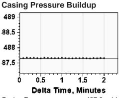
$\begin{array}{lll} \text{Casing Pressure} & 487.6 \text{ psi (g)} \\ \text{Buildup} & 0.0 \text{ psi (g)} \\ \text{Buildup Time} & 2 \text{ min 0 sec} \\ \text{Gas Gravity} & 0.6398 \text{ Air} = 1 \\ \end{array}$
