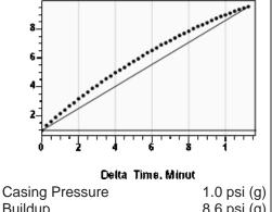
Buildup 8.6 psi (g) **Buildup Time** 11 min 15 sec Gas Gravity
