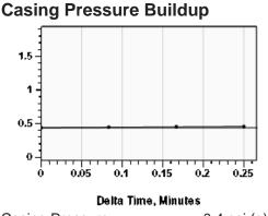
Casing Pressure 0.4 psi (g) Buildup 0.0 psi (g) Buildup Time 15 sec Gas Gravity 1.1618 Air = 1
