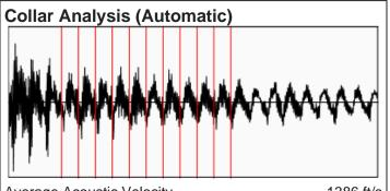
Average Acoustic Velocity Average Joints Per Sec. Joints To Liquid 1386 ft/s 21.86 Jts/sec 147.54 Jts
