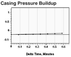
Casing Pressure -0.2 psi (g)Buildup 0.1 psi (g)Buildup Time 35 secGas Gravity 1.0270 Air = 1
