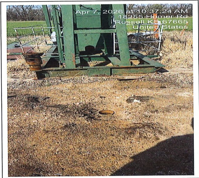
Weigel Oil Company Boxberger C 2 API 15-167-23135-00-00 SW NW SW SE 32-13S-14W 990 NSL 2324 WEL 38.87378 -98.89971 Casing on the Boxberger C 2 is open and uncovered.
