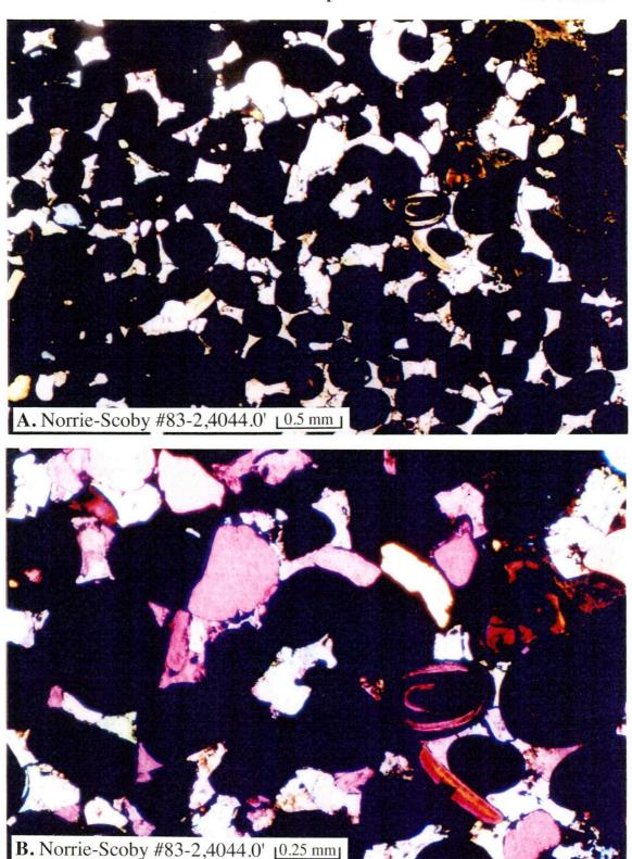
This sample was selected for petrographic study because it comes from a very heavy (dense) reddish-brown bed of ironstone a few feet thick with a distinctive log signature. The thinsection reveals that the rock is an oolitic ironstone with dolomite cement between the grains. Scattered grains of quartz sand and phosphatic fossil fragments are also present. The ooids are well sorted and appear to have formed as hematite.
