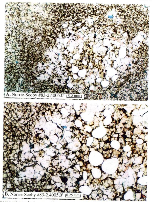
These photomicrographs show more of the same sample seen in Plate 1. They show another burrow containing sscattered superbly rounded quartz sand grains and minor calcite cement (stained pink) in a matrix of finely crystalline dolomite with some bitumen residue (dark brown) between the dolomite crystals. Also present are traces of pinpoint vuggy porosity (e.g., upper right, Photo A). Total visible porosity is less than 5% and reservoir potential appears poor.
