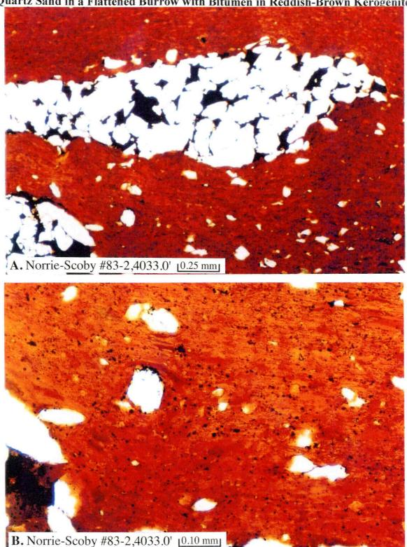
Shown here are more photomicrographs of the same kerogenite seen in Plate 8. A flattened burrow filled with quartz sand is visible in Photo A and scattered partly dissolved sand grains are visible in the reddish-brown kerogenite in Photo B. Ghosts of now flattened (but originally round) *Gloeocapsamorpha prisca* cells are visible in both photos. The nearly black material between the quartz sand grains in the burrow in Photo A is interpreted to be bitumen residue.
