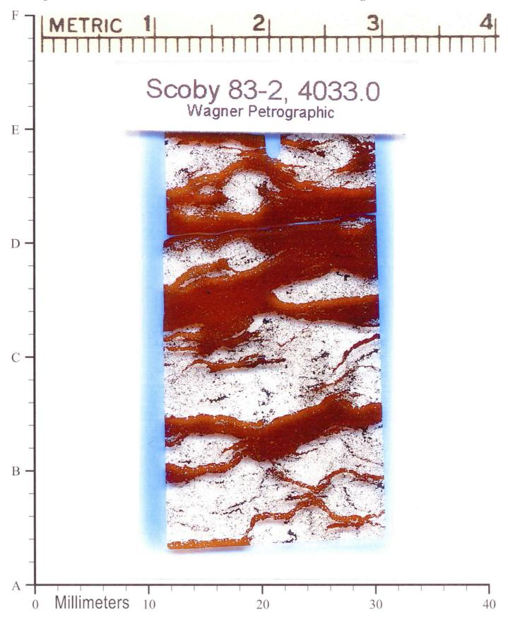
Interval: Simpson Group Sandstone Porous Bimodal Quartz Sandstone
