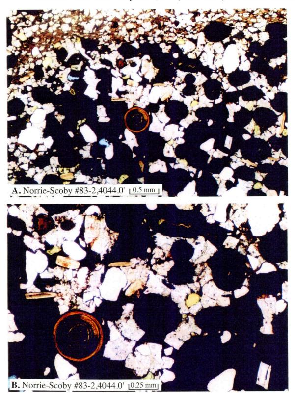
These photomicrographs show more of the same sample seen in Plate 13. An ooid with brown phosphatic bands is visible at lower left in Photo B (and near the center of Photo A), and the sample also contains scattered grains of yellowish glauconite (visible near the center of Photo B). A slightly shaly bed of siltstone is visible at the top of Photo A. Neither photo shows any significant visible porosity.
