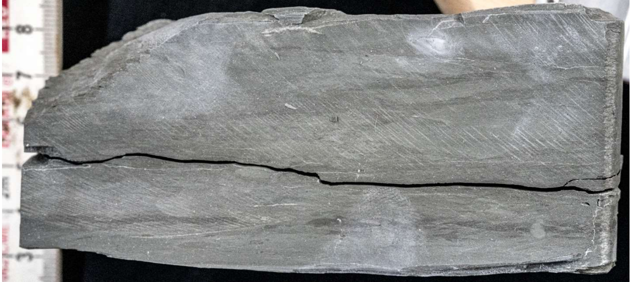
Figure 1. Green-gray medium-grained bioturbated mudstone at 1,839 ft of section. An underlying wavy non-parallel fabric is observable beneath planolites and chondrites burrows, which disrupt the original bedding. Note that a cm scale is placed in the background at the left side of the photograph.
