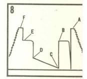
The packer has been unseated. testing assembly is being remo from the hole.
