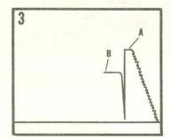
This chart shows the initial shut-in pressure. The methods by which this pressure can be taken allow only a minimum of formation fluid to be produced. This initial shut-in pressure is the best method yet devised for recording the original, undisturbed reservoir pressure of a formation.
