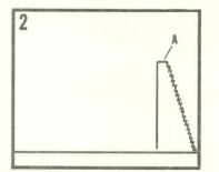
The packer is expanded and set to isolate the test zone. When the test valve is opened, a pressure drop is indicated on the pressure chart. This pressure drop is caused by removal of the hydrostatic mud pressure from the formation, allowing the formation to produce.
