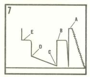
The chart shows the equalizing; the bypass ports have been opened permitting the drilling fluid to flow through the packer to the test zone. Thus, pressure is equalized above and below the packer. The equalization of the pressure facilitates easier removal of the packer from the packer seat.
