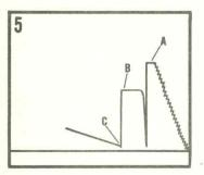
The pressure of fluid flowing from the formation into the well bore, through the perforated anchor, and into the drill pipe, is recorded on the chart.
