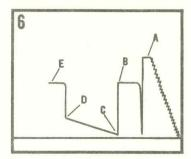
The final shut-in pressure is taken by stopping the flow of formation fluid into the drill pipe. Note the characteristic build-up curve. The well bore pressure is approaching equilibrium with the static reservoir pressure. When the shut-in curve levels-off the static reservoir pressure has been reached.
