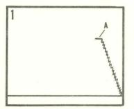
The pressure chart records the buildup in hydrostatic pressure as the test-ing assembly is lowered into the hole. Upon reaching the testing depth the hydrostatic head or pressure of mud column is recorded.
