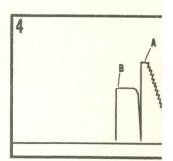
The chart indicates a pressure dr The test tool has been opened the surface either by breaking a d rotating a shut-in tool open or reopening the main testing valve permit the formation to produce.
