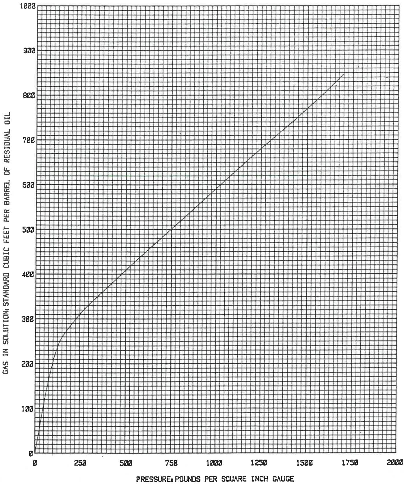
DIFFERENTIAL VAPORIZATION OF RESERVOIR FLUID AT 125 °F.
