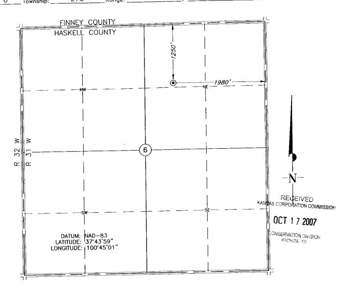
1000 1000 500 Topography & Vegetation: WHEAT Reference or Alternate Stakes Set: <u>NONE</u> GRAPHIC SCALE IN FEET (1" = 1000") Best Accessibility to Location: FROM LEASE ROAD EAST OF LOCATION Distance & Direction: \_\_\_ ±22 MILES NORTHEAST OF SUBLETTE, KANSAS
